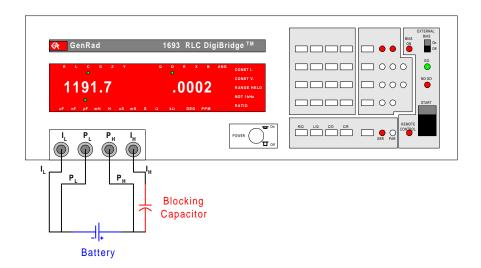
For faster and more accurate testing, build a test fixture and mount the blocking capacitor in this test fixture. The test fixture should provide four terminal connection to the digibridge instrument. A 1689-9602 4-BNC to 4-BNC test cable can be used to connect the fixture to the instrument when using a 1689M, 1693, 1710 or 1750 Digibridge.
